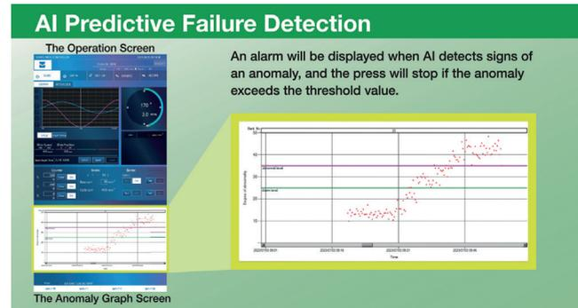
*\*The press operation will pause if the anomaly exceeds the threshold value.*
