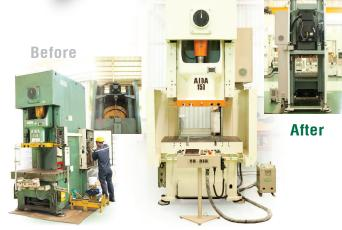
Modernization including upgrade from mechanical press to servo press. To reduce chances of malfunctions, enhance safety & to increase productivity performance.
