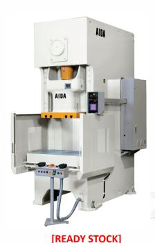
Capacity 800kN Die Height, Slide To Bolster 320mm 160mm Stroke Length **Bolster Thickness** 140mm Slide Adjustment 80mm **Bolster Height** 900mm 40~75mm Stroke Per Minute Slide Area (L.R X F.B) 540 X 460mm **Bolster Area (L.R X F.B)** 950 X 600mm 310mm Frame Gap Max Upper Die Weight 203kg Main Motor (Variable Standard) 7.5kW **Power Supply** 380v,50Hz **Required Air Pressure** 0.5Mpa Approx. Press Weight 6.0ton **Exterior Color** 5GY 9/1
